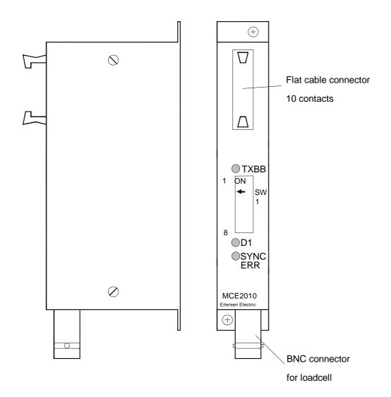
The loadcell modules are connected to each other using the supplied cable (10 pole ribbon cable). The terminal module (the one with connection terminals) and possibly a communications module are connected using the same cable.
