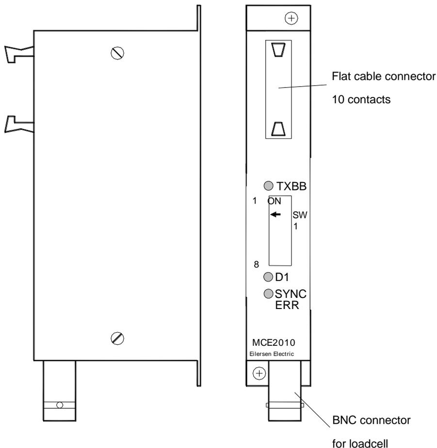
The load cell modules are connected to each other using the supplied cable (10 pole ribbon cable). The MCE9601 terminal module (the one with connection terminals) and the MCE2035 Profibus-DP module are connected using the same cable.
