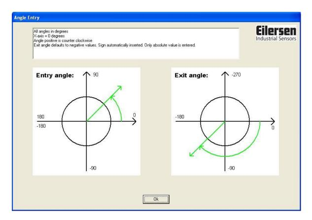
The terms *Entry* and *Exit* angle are chosen arbitrarily and can be switch for convenience. **Please be careful** when angles from machine drawings are used. They **must** be recalculated to fit the above definitions before used in the software.
