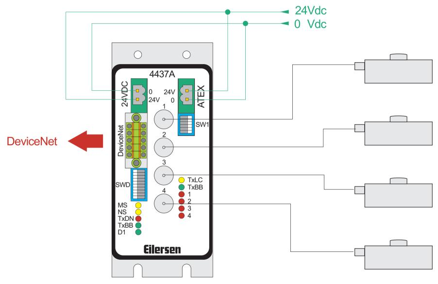
BNC connectors for load cells
