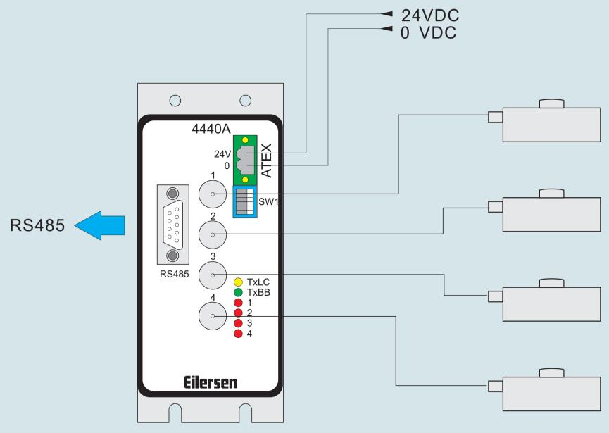
BNC connectors for load cells
